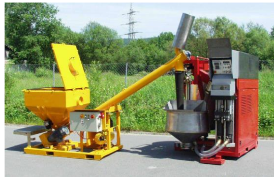
VS 109-D with option Proportioning auger type FS-DKB 160 D for silo cement and bag material
